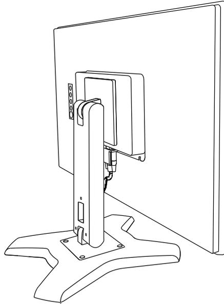
2. After connecting the cables to the monitor, use the cable management slot to organize all cables shown below.
